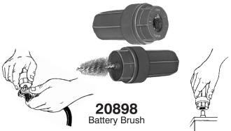
Cleans dirt and corrosion from post type battery terminals and cable clamps. Made of heavy duty stainless steel wire. Case is made of high impact plastic that will not weaken in cleaning solutions.
