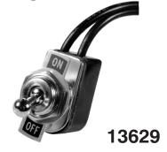
S.P. S.T. Toggle Switch -"Off-On" Two 6" Wire Leads. With nickel plated "Off-On" indicator plate assembled. Mounting stem 3/8" long. 15/32" diameter. Bat handle. 15 Amps 12 Volts DC Rating: 6 Amps 125 Volts AC
