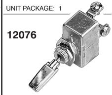
Heavy Duty Toggle Switch 2 position "On-Off" For 35 Amp. 6-12 Volt DC. 15/32" Stem Diameter. Low Voltage -High Amp Application. Chrome Plated Handle.
