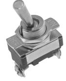
S.P. S.T. Toggle Switch -"Off-On" Phenolic housing. Mounting stem 15/32" long; 15/32" diameter. 2 screw terminals. Bat handle Rating: 15 Amps 125 Volts AC 10 Amps 250 Volts AC
