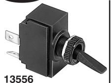
Toggle Switch 2 positions "On-Off" For lights, blower, pump, etc. Black plastic paddle and locking ring with level seal and knurled cap nut. Sealed to resist water penetration. Fits panels up to 1/4" thick; requires 15/32" mounting hole. Rated 20 Amps @ 12 Volts D.C. and has 1/4" spade terminals
