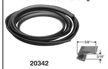
A universal windshield rubber moulding for domestic and import vehicles. Made of EPDM rubber, this moulding contains a butyl bead that adheres to the glass during installation. The profile design allows for the moulding to attach easily to the glass edge and lay evenly on the vehicle body along straight areas and around corners.
