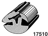
Glass Thickness: 1/4" Body Thickness: 1/8" Self-Locking Type
