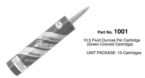
For use as a water and dust seal on exterior and interior body surfaces. New improved formula allows for a longer open time so it can be tooled for several minutes after being applied. Cures to a firm abrasion resistant seal with no cracks or peeling. Can be air dried or force dried and then painted within 30 minutes
